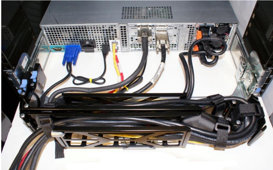
Figure 5: Left-Side Mounted CMA Installation (Preferred)
